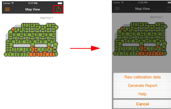
Figure 69. Click the Options icon to access the Help, Generate Report and Raw Calibration Data tools
